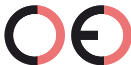
False CE Mark (too far)
